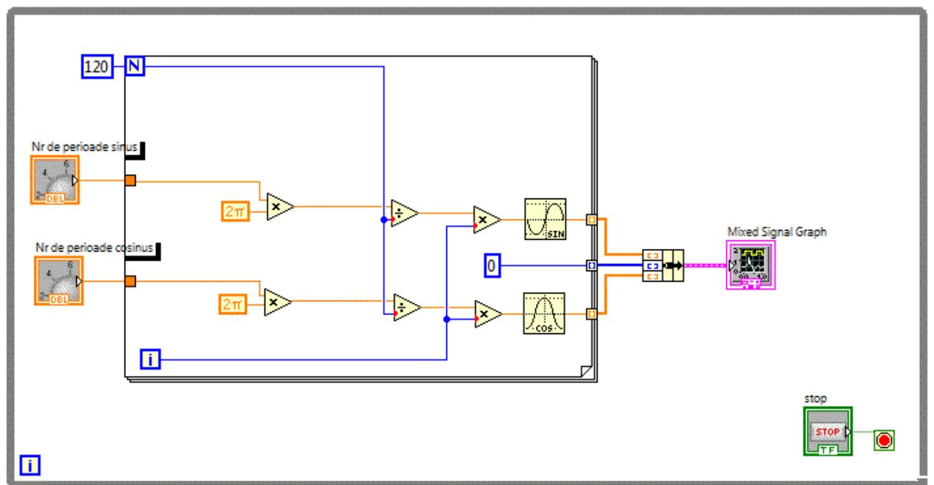
Putem folosi o functie Simulate Sig aflata in: Function->Programming->Waveforms->Analog Wfm->Generation->Simulate Sig care genereaza diverse forme de unda
